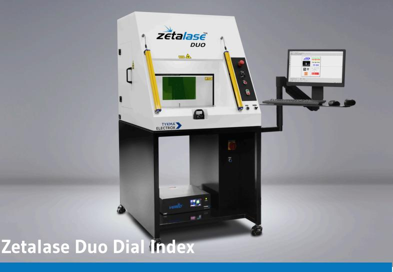
Ideal for high volume marking, the Zetalase™ Duo dial index system allows the operator to load/unload parts while others are being marked. The addition of safety light curtains ensures operator safety. Our Zetalase Duo workstation utilizes a robust, high duty-cycle rotary indexer for years of trouble free operation. Custom holding fixtures can be engineered for a variety of applications.
