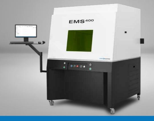
With the ability to run up to four axes, EMS400 is ideal for large tray and part marking. EMS400 features an automated 24" x 24" XY stage (610mm x 610mm), ideal for marking trays of parts or large components in multiple locations. A front vertical pneumatically actuated door maximizes operator ergonomics.
