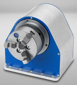
The ZD30 is a compact, rugged rotary axis incorporating a stepper motor with a play-less timing belt and is capable of a 100% duty cycle operation. ZD30 has a 15mm diameter through hole allowing longer components to be marked. When sold independent of a laser or workstation, the ZD30 is supplied with drivers, power supplies and a limit switches.
